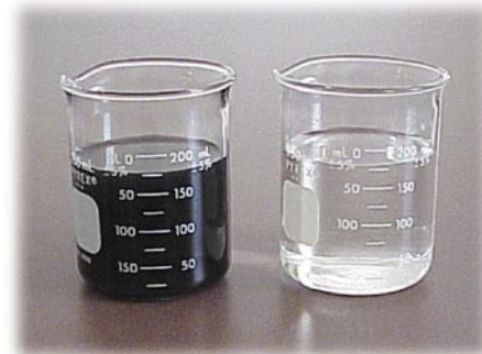
Figure 4 Dirty Caster Water (left), Clean Filtrate (right)
